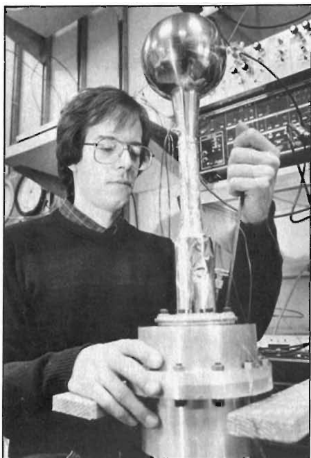
Tom Hofler attaching the resonator of the cryocooler to the housing of the cooler's driver and hot heat exchanger.
